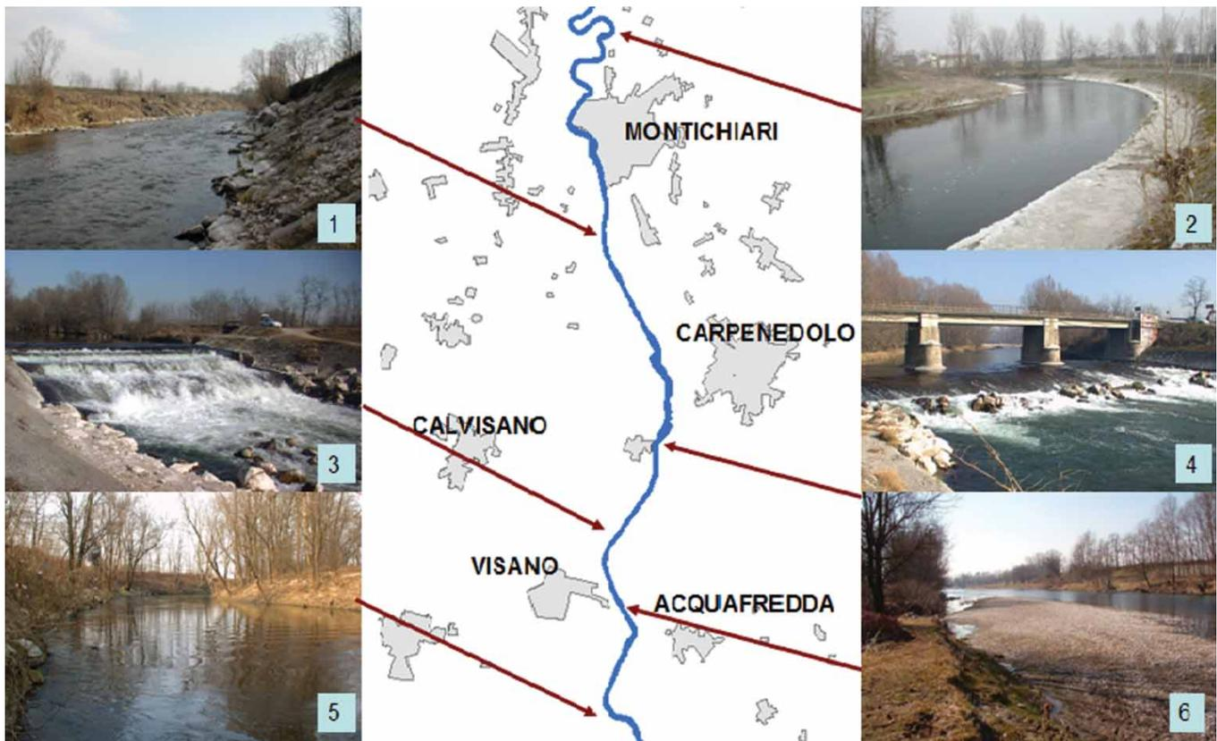
Figure 2 Examples of engineering structures along river Chiese. (1) Rectified reach, now sensibly incised downstream Montichiari, characterized by high levees and extensive bank protection; (2) concrete bank protection in a meander bend upstream Montichiari; (3) one of numerous barrages for irrigation purposes; (4) bridge downstream Carpenedolo protected from erosion by a rocky bed sill; (5) and (6) quasi-natural cross-sections near Acquafredda
