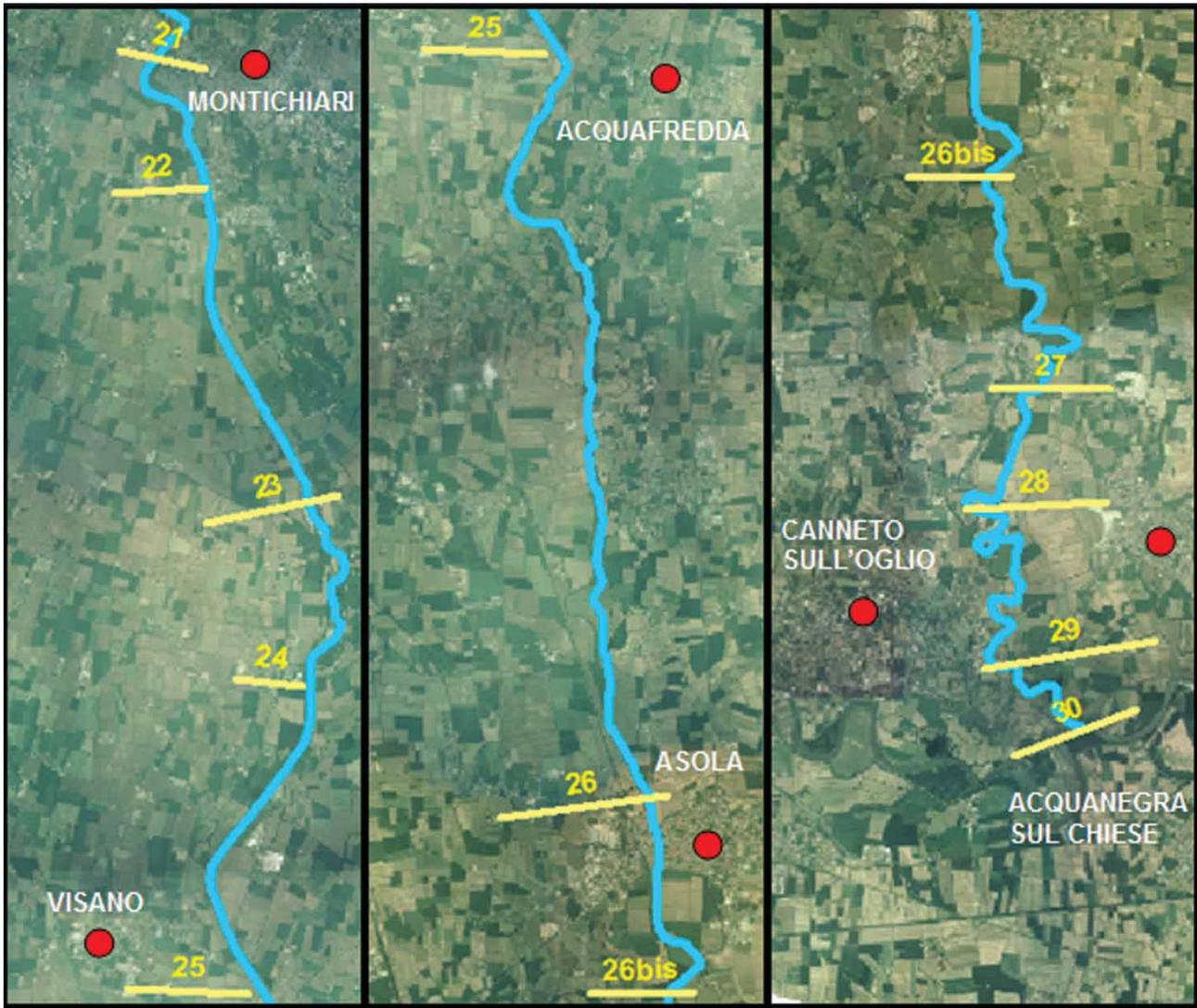
Figure 4 Identification of geomorphic homogeneous river stretches of lower Chiese River (left: upstream; right: downstream). The identifier of a Stretch is located at its head (the last one represents downstream boundary conditions)
