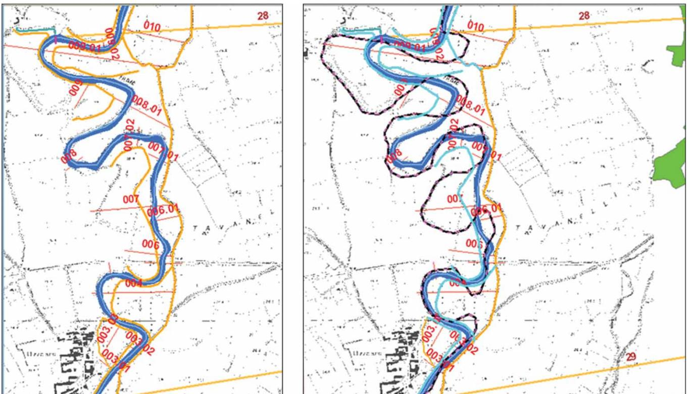
Figure 9 Example of planform prediction (ALT\_Base, stretch 28; see Figure 8 to locate it). In this figure, the light brown lines along the river indicate works that exist and will stay in the considered *alternative* ALT\_Base, while the light blue ones indicate works to be dismissed. The new planform is the dashed violet-black, thick meandering line (on the right)
