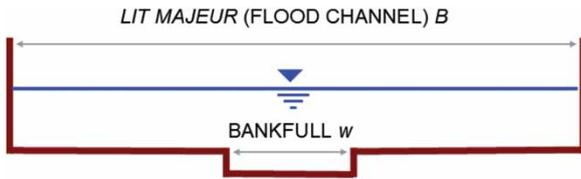
Figure 8 Cross-section schematization as a double rectangle
